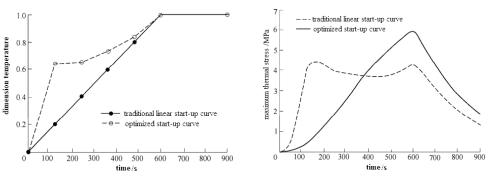
(a) Dimensional temperature-time (b) Maximum thermal stress-time
