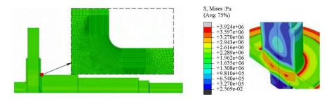
Figure.2 Schematic diagram of mesh generation Figure.3 Distribution of maximum thermal stress (120th second)
