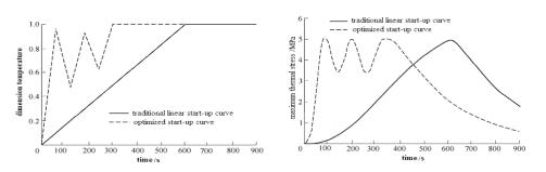
(a) Dimensional temperature-time (b) Maximum thermal stress-time
