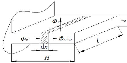
Figure. 2 1/2 model of fin heat conduction
