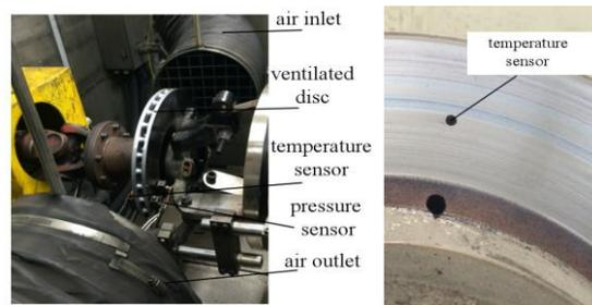
**Figure.5** The ventilated disc and related sensor installation diagram
