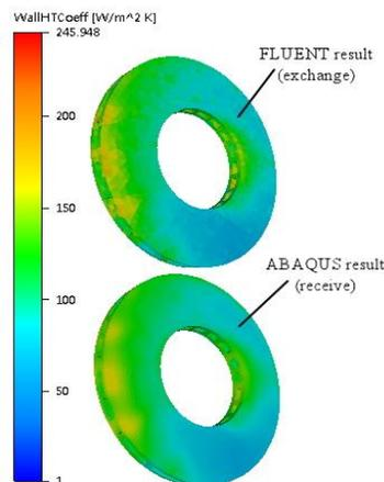
(c) Surface heat transfer coefficient
