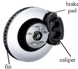
**Figure.1** Structure diagram of ventilated dis
