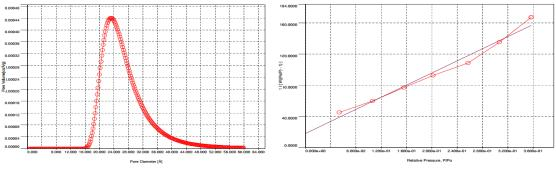
Volume of porous hole = 0.005 cc/gPorous hole diameter = 2.320e+01 Å
