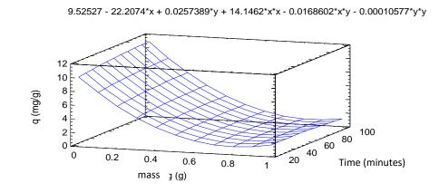
**Figure 3.** The interaction effect between mass of the adsorbent and adsorption time to the MB adsorption capacity of rice husk ash.
