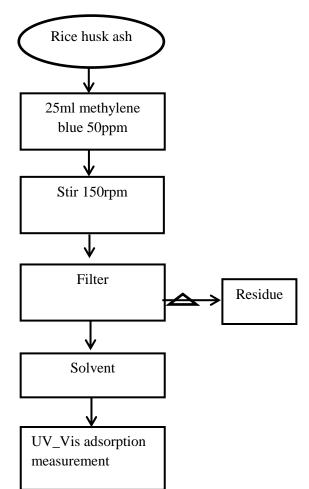
**Diagram 1.** The experimental procedure to investigate the influence of pH, rice husk ash mass and adsorption time to the MB adsorption capacity of rice husk ash
