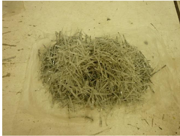
Picture 9. Plastic flakes break down once compressed beyond 32 kN
