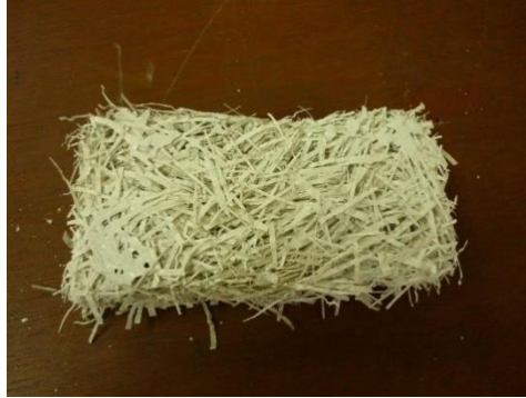
Picture 6. A 160 g brick out of plastic waste
