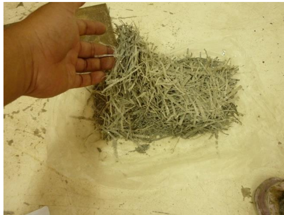
Picture 8. Plastic waste bricks when compressed by 29 to 32 kN
