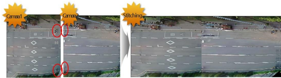
Figure 3 Image stitching using maker point
