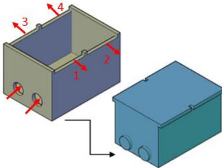
Figure 1. Geometry of the distribution chamber (left) and water volume (right)
