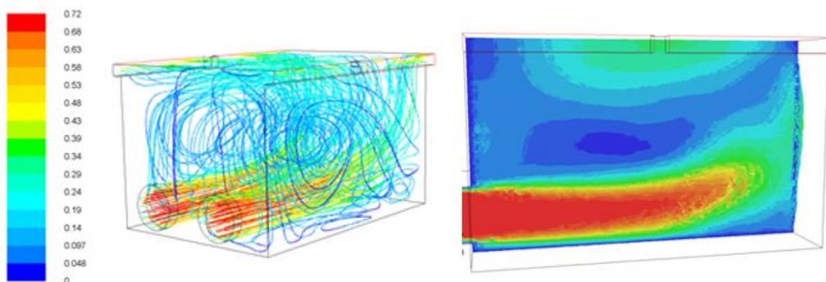
Figure 2. Pathlines in the distribution chamber (left), filled velocity contour lines at a section (right). Coloured by velocity with the scale of m/s.
