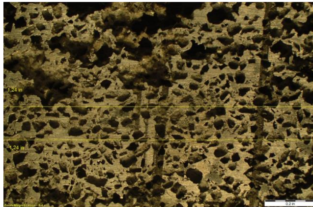
Figure 4.(a) Samples from which the NaCl grains were dissolved and the surplus aluminium that was not infiltrated was removed. (b) Photograph of one of the samples of open cell metal foam, which have been sectioned, polished and observed under an optical microscope at 4x.
