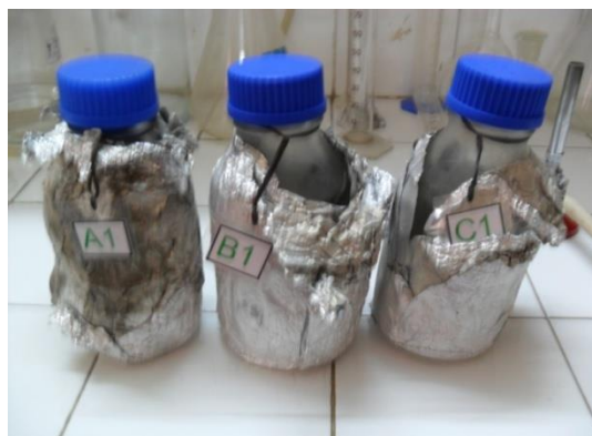
Photo 2: 250 ml sterilized glass vials coated with aluminum foil to collect water
