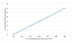
Figure 12. Graphic of correlation between pedal angle with the current of servo motor
