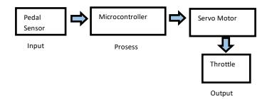
Figure 6. Block diagram of *throttle by wire* system
