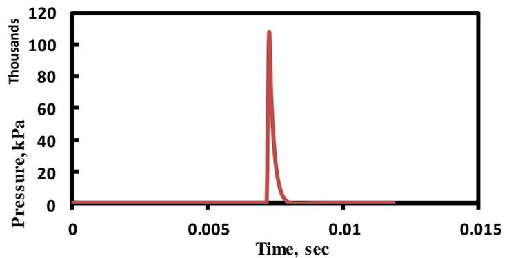
Figure (8): The incident wave due to detonation of 100 kg TNT
