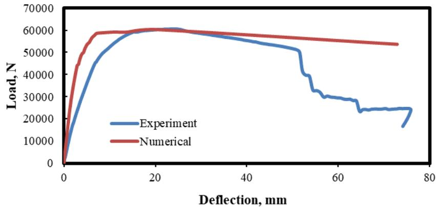
**Figure (10):** Vertical load- deflection relationships at middle column
