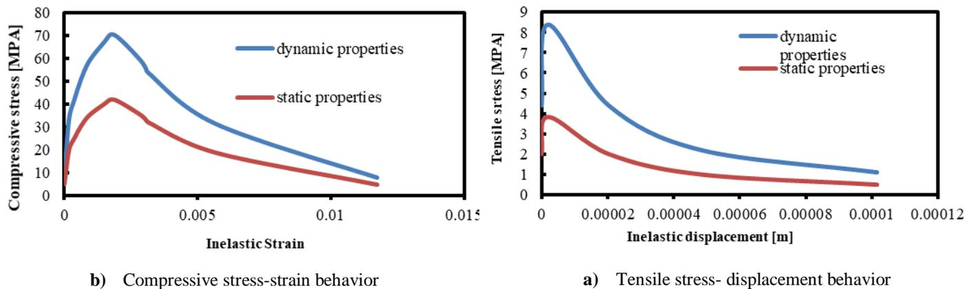
**Figure (6):** The compressive and tension behavior at static and dynamic load.
