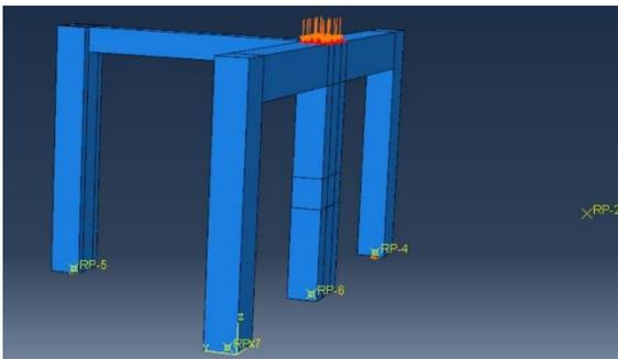
Figure (7): The applied load and source of detonation
