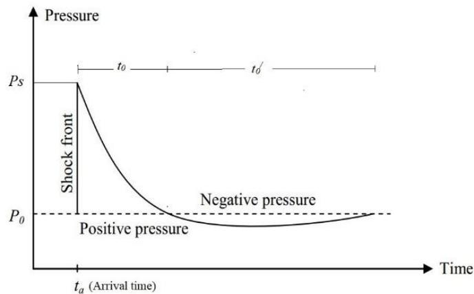
**Figure (1):** Pressure-time profile of the explosion wave
