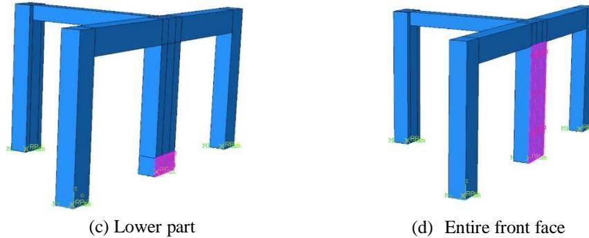
**Figure (5):** Different locations of application of explosion load on the middle column
