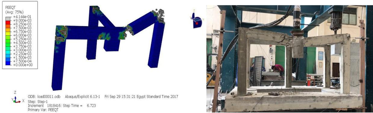
**Figure (9):** Modes of failure in both experimental and FE model (1)
