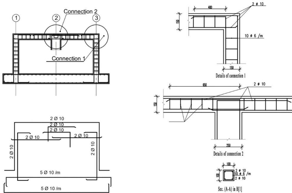
Figure (3): Reinforcement detailing of the studied frame (Dimensions in mm)
