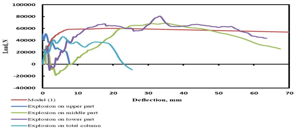
**Figure (11):** The load- deflection relationships at middle column due to Explosion load
