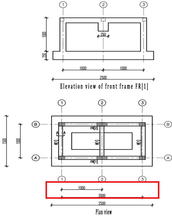
Figure (2): Dimensions of studied frame (Dimensions in mm)
