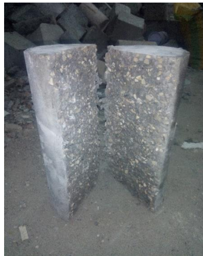
Figure 3 Sample of Brazilian tensile test
