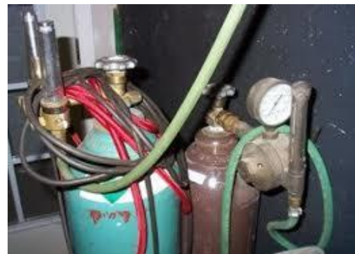
Figure 2: shielding gas cylinder and regulator
