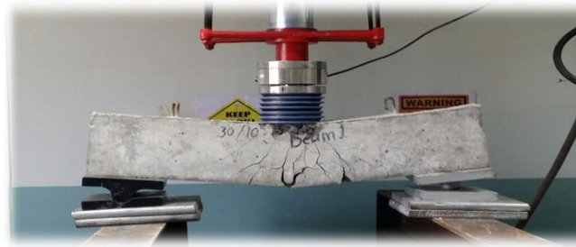
Figure 9 Beam B1 after Failure
