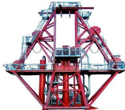
Fig.2 Semi-Active Heave Compensator
