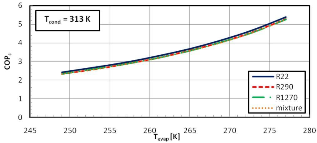
Figure 11: COP of R22, R290, R1270 and R290/R1270 mixture at different evaporator temperatures
