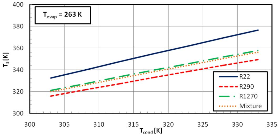
Figure 16: Compressor exit temperature of refrigerant of R22, R290, R1270 and R290/R1270 mixture at different condenser temperatures
