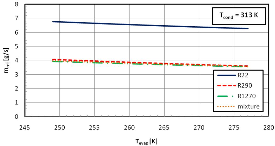
Figure 7: the mass flow rate of R22, R290, R1270 and R290/R1270 mixture at different evaporator temperatures
