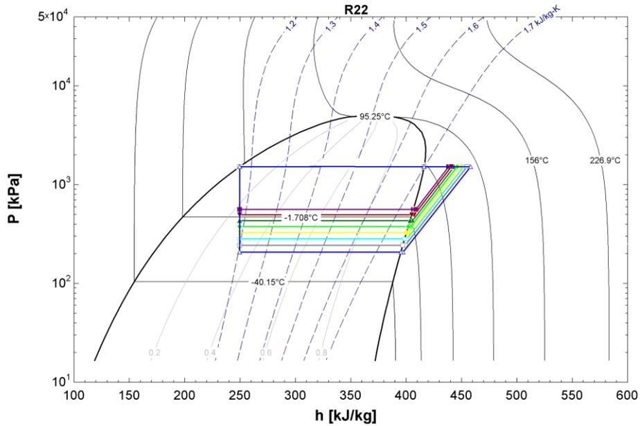
Figure 6: p-h diagram of a simple refrigeration cycle using R22 at different evaporator temperatures and the same condenser temperature
