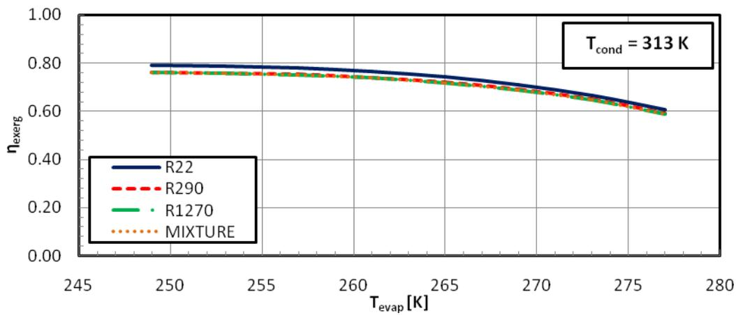
Figure 12: The exergetic efficiency of R22, R290, R1270 and R290/R1270 mixture at different evaporator temperatures
