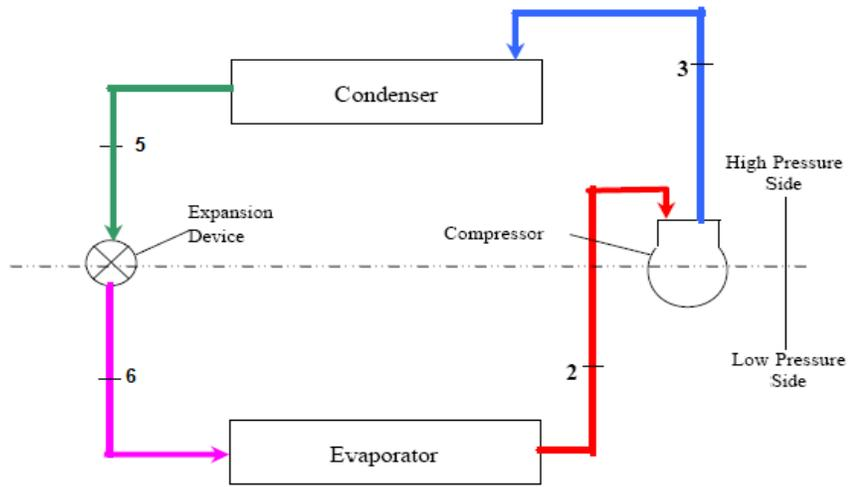
Figure 5: Schematic sketch of the cycle
