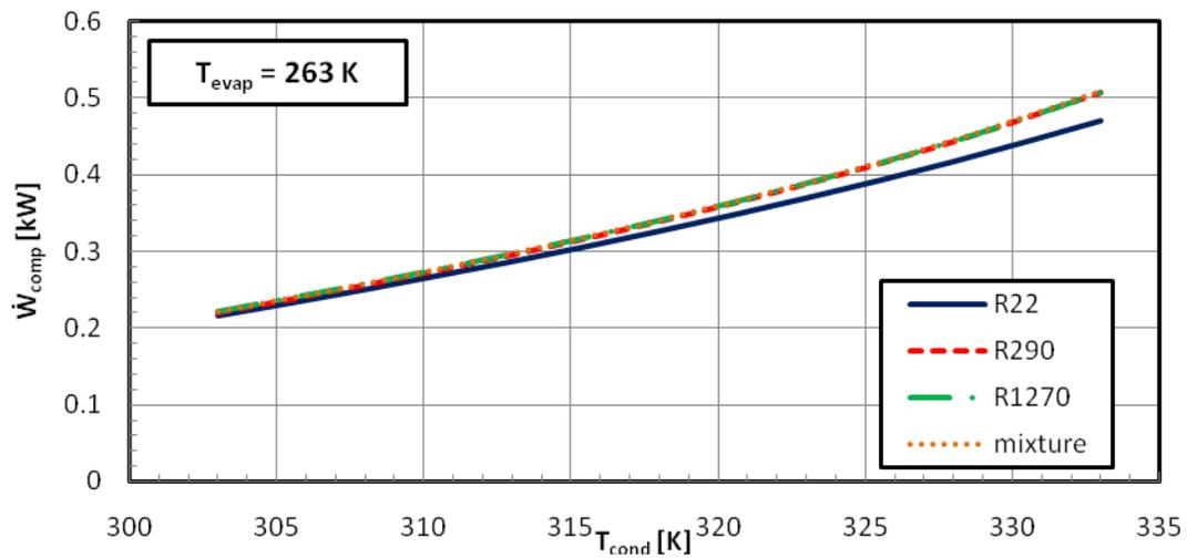
Figure 17: Compressor power consumption of R22, R290, R1270 and R290/R1270 mixture at different condenser temperatures
