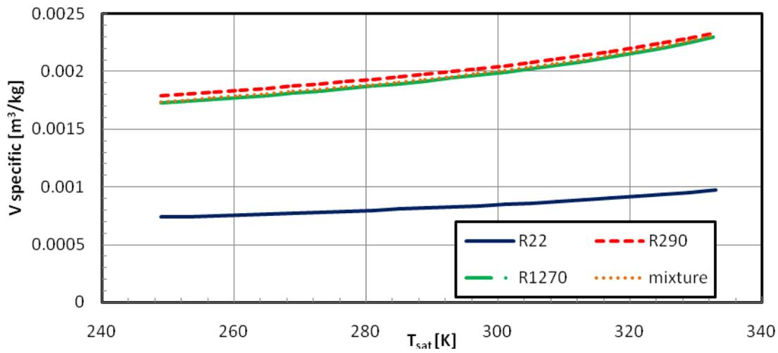
Figure 1: Specific volume of saturated liquid at different temperatures
