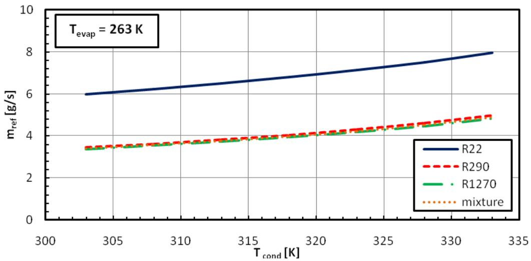
Figure 14: The mass flow rate of R22, R290, R1270 and R290/R1270 mixture at different condenser temperatures
