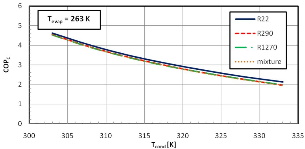
Figure 18: COP of R22, R290, R1270 and R290/R1270 mixture at different condenser temperatures
