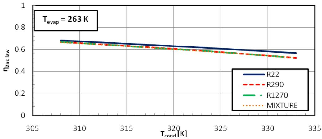
Figure 20: The second law efficiency of R22, R290, R1270 and R290/R1270 mixture at different condenser temperatures
