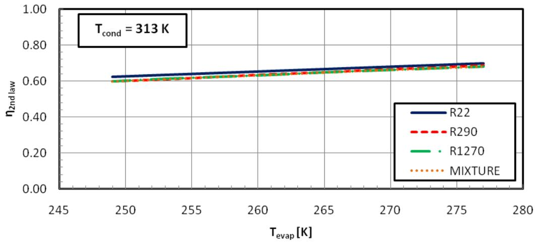
Figure 13: The second law efficiency of R22, R290, R1270 and R290/R1270 mixture at different evaporator temperatures
