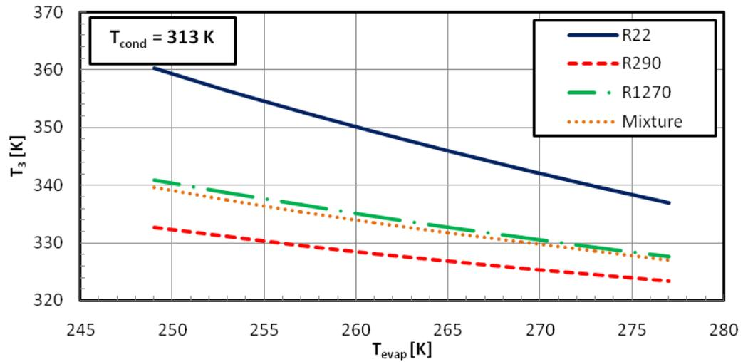
Figure 9: The compressor exit temperature of R22, R290, R1270 and R290/R1270 mixture at different evaporator temperatures
