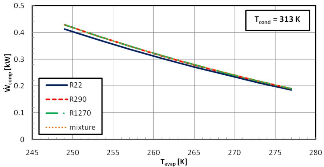
Figure 10: The compressor power consumption of R22, R290, R1270 and R290/R1270 mixture at different evaporator temperatures
