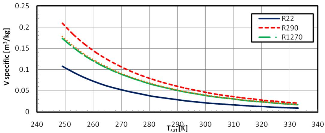
Figure 2: Specific volume of saturated vapor at different temperatures
