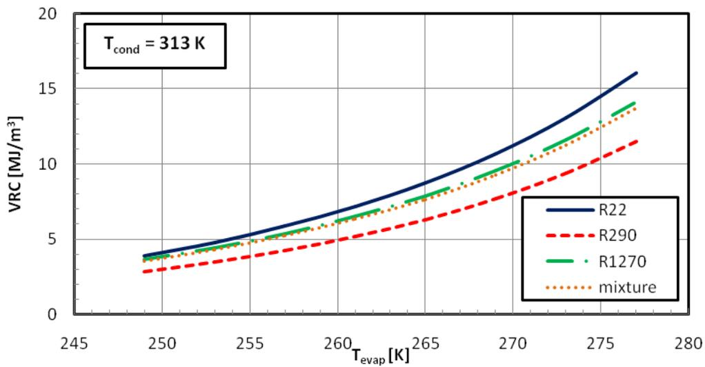
Figure 8: VRC of refrigerant of R22, R290, R1270 and R290/R1270 mixture at different evaporator temperatures
