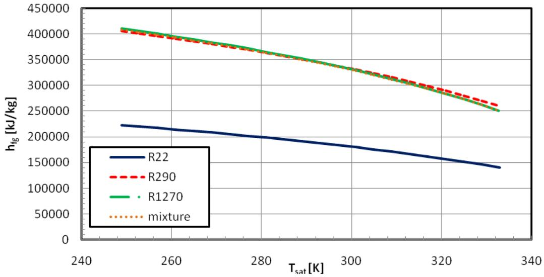
Figure 4: The variation of the latent heat of refrigerants with saturation temperatures
