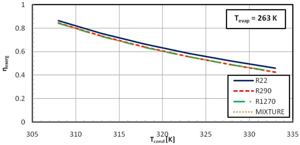
Figure 19: The exergetic efficiency of R22, R290, R1270 and R290/R1270 mixture at different condenser temperatures
