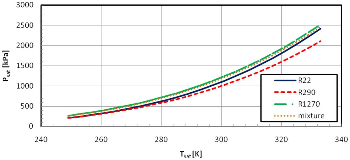
Figure 3: The variation of saturation pressure of refrigerants with the temperatures
