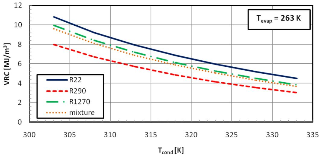
Figure 15: VRC of refrigerant of R22, R290, R1270 and R290/R1270 mixture at different condenser temperatures
