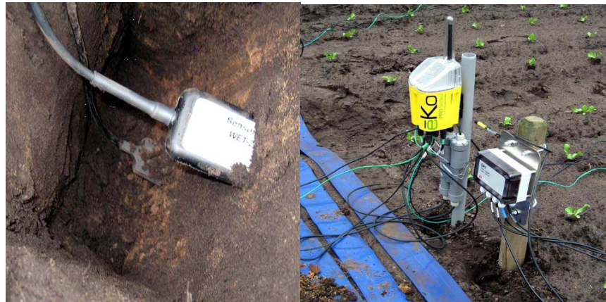
Figure 5 A WET-sensor (Delta-T-Devices, UK) and a 5TE (Decagon, US) to measure water content, EC and temperature (left); a wireless sensor network (eKo,Crossbow, US) and irrigation controller (GP1, Delta-T Devices, UK) (Balendonck et. al., 2010).
