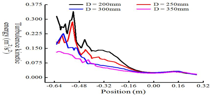
c Turbulence kinetic energy
