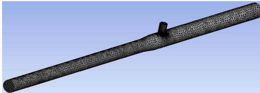
Figure 2 Finite element model
