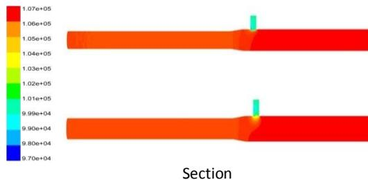
Figure 3 Static pressure nephogram
