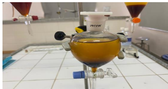
Figure 4. Crude biodiesel obtained using batch reaction.
