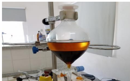
Figure 5. Biodiesel from reactive distillation column.
