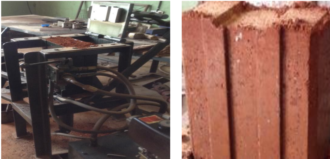
Fig. 1: Semi-Automated Interlocking Block Making Machine, SAIBM and the block (Diesel Generator Driven)
