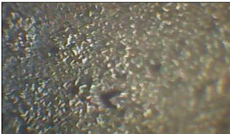
Plate III: DCEP E 1 HAZ at X 400
