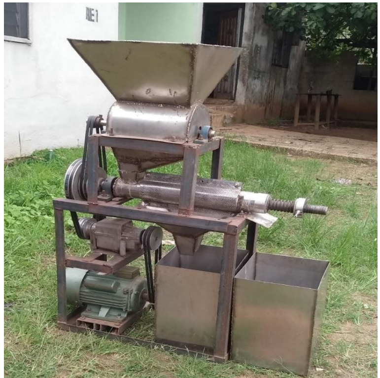
Plate 1: Cassava processing machine
