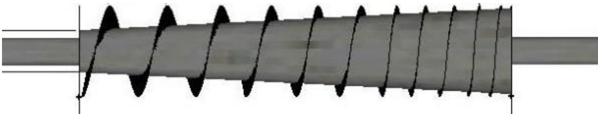
Fig. 2: The screw expeller
