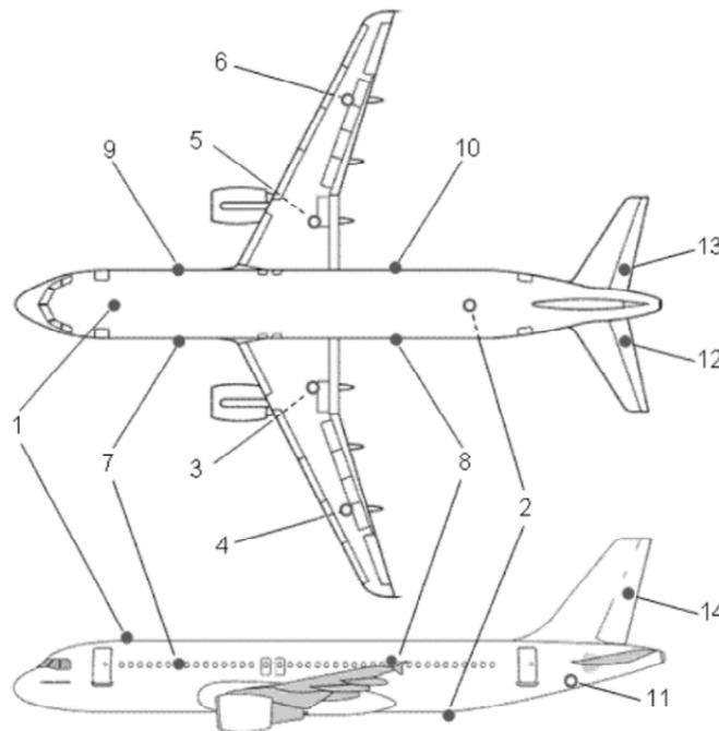
Figure 1. Sensors on the aircraft (Sensor locations, online): 1 – Fuselage; 2 – Housewheel steering sensors; 3, 5 – Trailing edge flaps; 4, 6 – Spoilers; 7, 9 – Front cabin; 8, 10 – Rear cabin; 11 – Tailplane; 12, 13 – Elevators; 14 - Rudder
