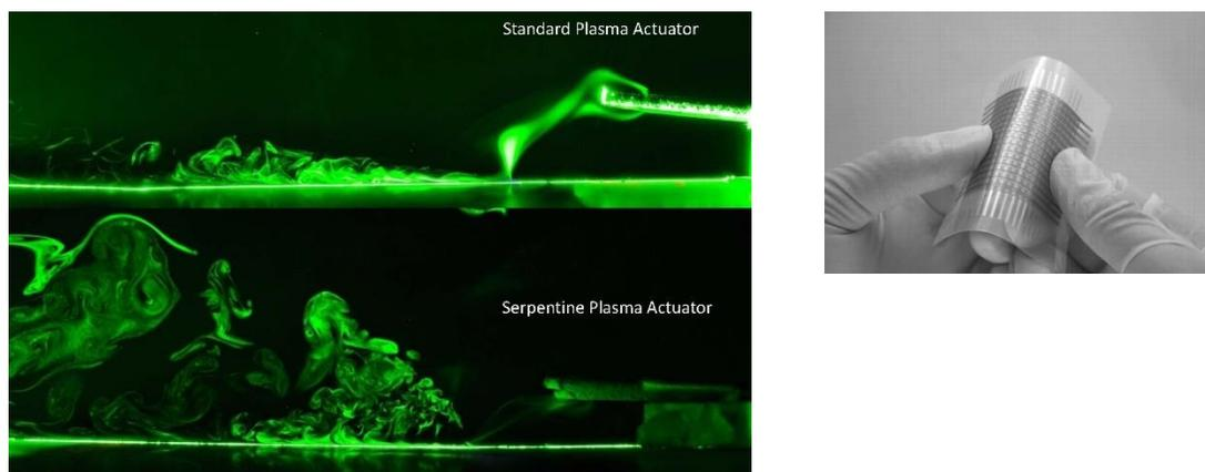
Figure 2. DBD Actuators (DBD Actuators, online) (left) and A large-area, flexible pressure sensor matrix (Someya, Sekitani, 2004) (right)
