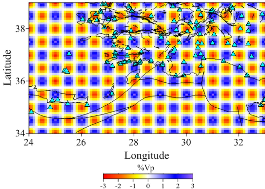
Figure 8. The initial checkerboard synthetic model is for P-wave data. For each grid node, the positive and negative synthetic velocity perturbations ( $\pm 3\%$ ) denote with red and blue colors respectively. The seismic stations are shown with blue triangles. The solid lines show active faults.
