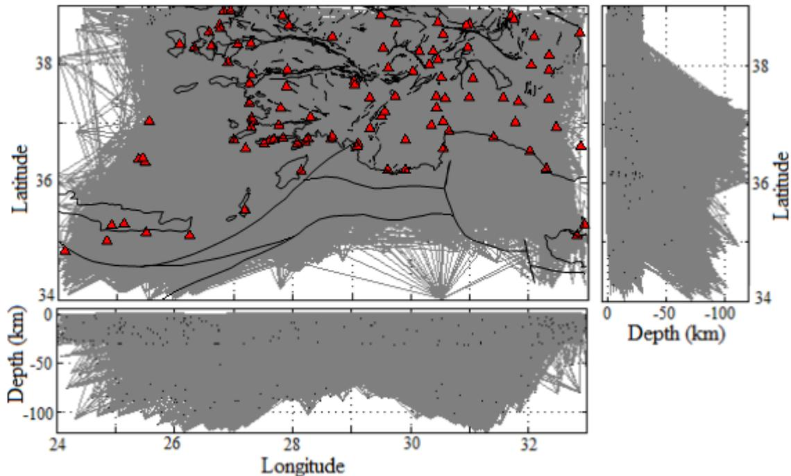
Figure 5. The ray-path coverage of P-wave data set. The paths are drawn as a straight line from focal of earthquake to the station.
