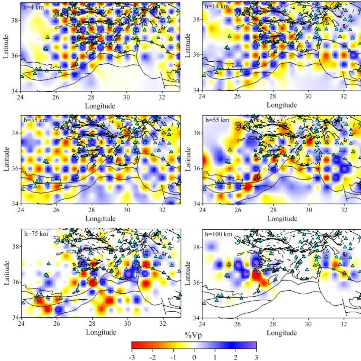
Figure 9. The results of checkerboard resolution test at six depths of 4-, 14-, 35-, 55-, 75- and 100-km. The high and low velocities are shown with red and blue colors respectively. The solid lines show active faults.
