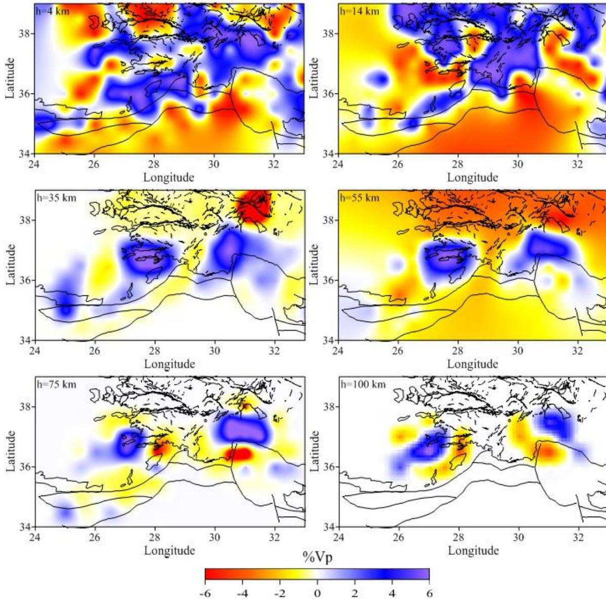
Figure 10. P-Wave velocity values (in %) at six depths of 4-, 14-, 35-, 55-, 75- and 100-km. The solid lines show active faults.
