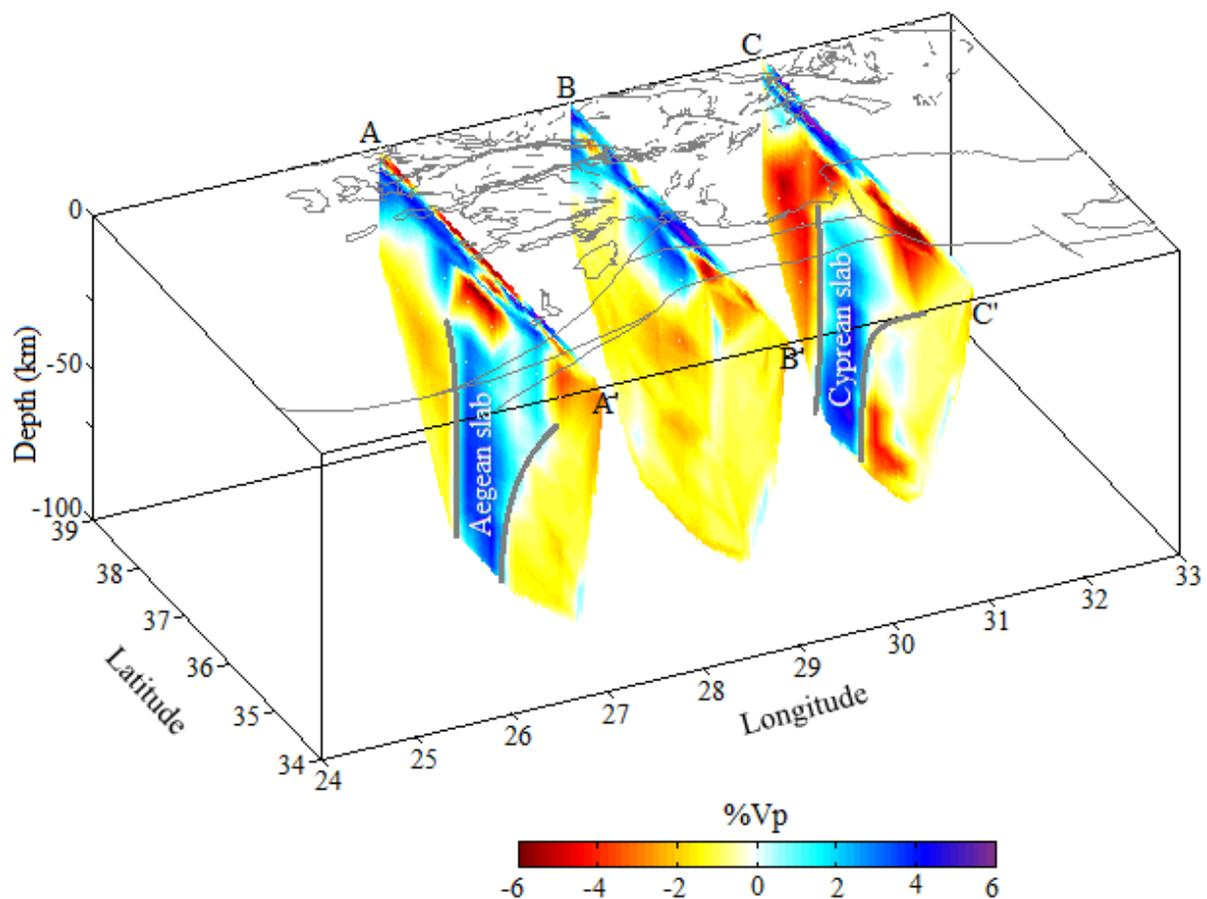
Figure 11. It is the block diagram of the vertical cross sections of Vp % along lines AA', BB' and CC' configured as N-S direction shown in Fig. 6. The red color denotes high, blue color denotes the low Vp % values.
