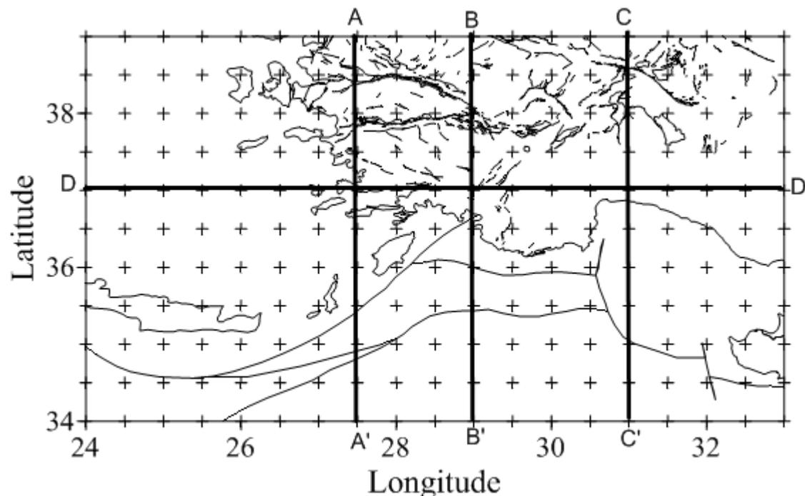
Figure 6. It is the grid net configure to the study region in horizontal spacing as  $0.5^{\circ} \times 0.5^{\circ}$ . The vertical cross-sections are shown with the straight lines. The active faults are shown by thin lines.
