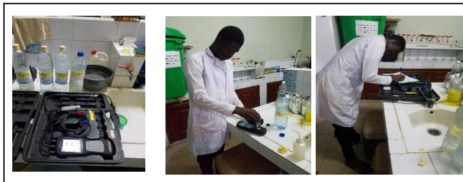
Plate 2: a HORIBA and COLORIMETER type device for the analysis of pH, CE, temperature, TDS and Turbidity
