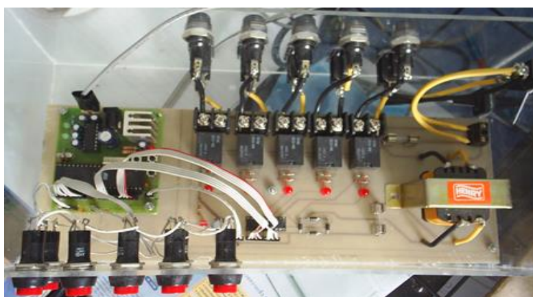
Figure 6. Relay Control Circuit Hardware Kit
