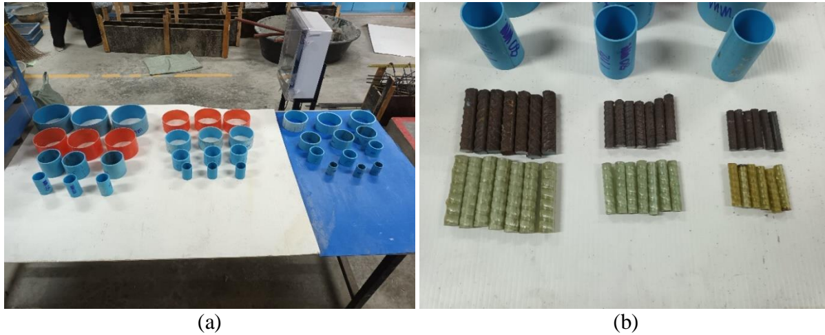
Figure 2. Specimen: (a) PVC cases and (b) GFRP and steel bars.
