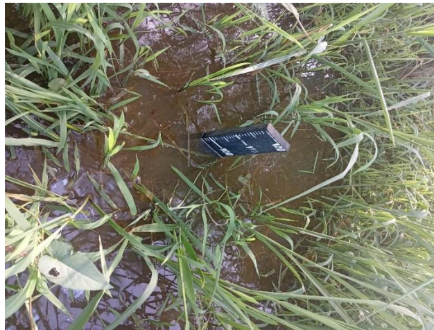
Photo 2: Limnimetric scale on the Grand axis-Popo Comé Shooting: Maboulou, June 2026
